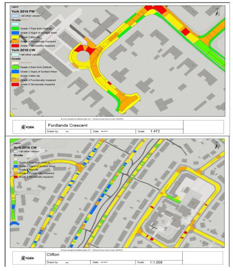
The survey information has measured the dimensions of the entire network and is able to identify the current construction type of the footway or carriageway.
